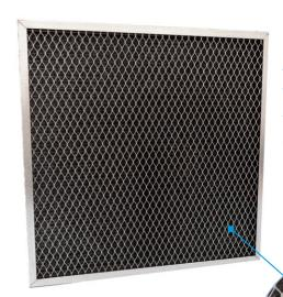
Galvanised or stainless steel outer frame construction provides rigidity and longevity. The central section of the filter frame contains two channels which accept two mesh screens of varying density. These screes can be withdrawn from the filter frame for cleaning by vacuum, pressure washer, scrubbing, etc. and then replaced for continued filtration performance.
